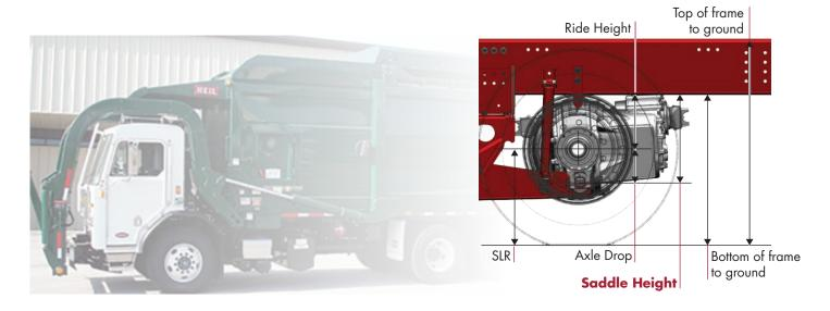
Examples: How the Saddle Height can affect the Ride Height and Frame Heights in different vehicle configurations and operating conditions. (shown for 16.5" Saddle Height)
