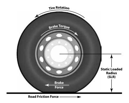
The charts below summarize standard on-highway trailer tire sizes and the typical static loaded radius (SLR) for trailer tread patterns. Please consult the tire manufacturer for the exact SLR for the size, tread and load range of your specific tire.
