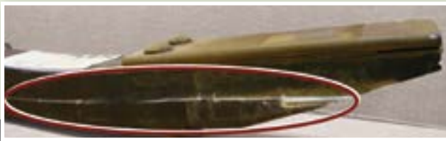
Side to side crack extending beyond 75% of the length of the spring
